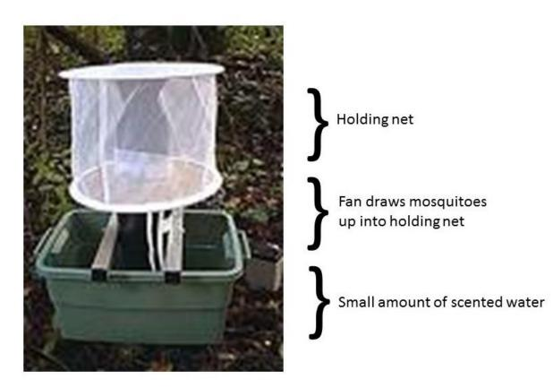
Fig. 1. Components and set-up of a gravid trap
